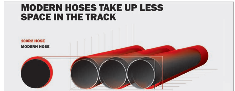
Fig. 5: Reduced size of hose and required guide track.
