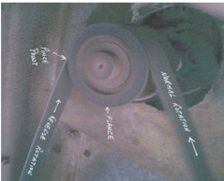
Belt and pulley form a pinch point that can trap and sever fingers.
